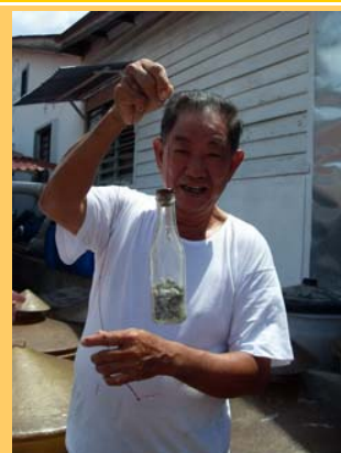
Mr. Baey, the Founder showing us how to gauge the consistent of salt water by using a bottle which filled with small stone.
